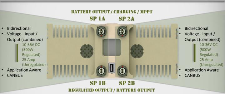
Smart Ports 1A & 1B are tied together. One can output Regulated Power while the second one outputs Battery (Unregulated) Power when operated simultaneously. Same is the case for Smart Ports 2A & 2B.
